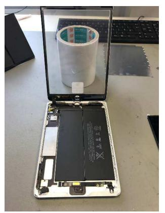
We can now fit the new screen onto the device. I use my lens tape to hold the screen up. I'll always use something to hold the screen up as we'll need to fit the LCD next.
