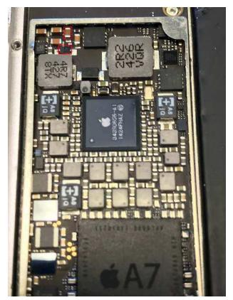
With this metal plate removed we can locate the capacitor and diode. The brown component that is highlighted is the capacitor. This had blown at some point. Causing the diode which is also highlighted to blow also.
