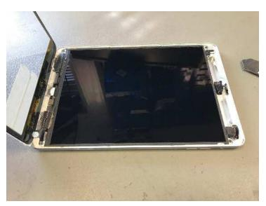
This is how the screen will come away. Make sure to be cautious when lifting screen away near the home button. As there is 2 thin flat flexes that may stick to the screen.
