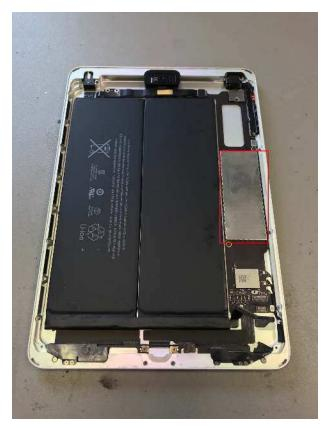
Due to the backlight being blown we needed to take a look at the capacitor that controls the backlight and see if it's killed the capacitor and needs replacing.
