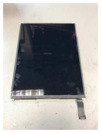
Secondly we'll check the LCD, making sure there has been no damage during removal. If there is no damage, we'll go forward and check there isn't any glass shards that are going to cause some scratches when we move the component about.
