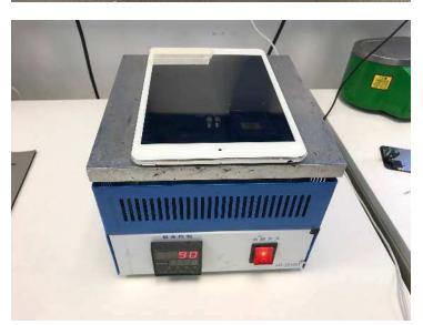
The heat plate is set to 90. At this temperature we can leave the device on here a long as we want, without having to worry about causing any damage.
