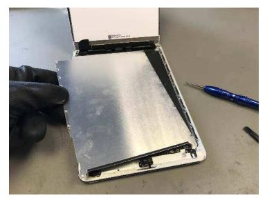
Once the screws are removed the plate will lift up and slide out.
