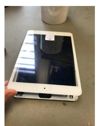
With all dust removed we can now fit the screen down.
