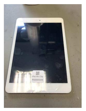
With the screen fitted, again we'll give it a check over before we tape the device up. Making sure it fits down properly and no dust or anything else is in between the LCD and Digitizer.
