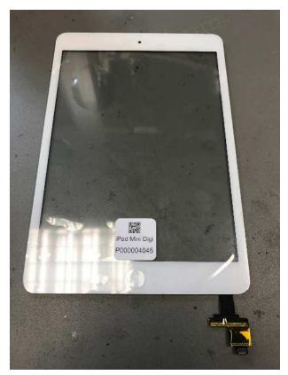
Before attempting to fit the new screen, it's always best to give the part a quick check over before fitting. Making sure there is no scratches, cracks or any marks that will affect the fitting or look of the device.
