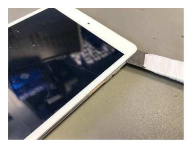
Once the device is heated up. We'll use a flat metal pry tool (Sesamo Tool) to get in between the digitizer and frame.
