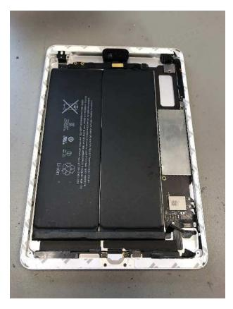
With the hard part done we can now fit the metal plate back on and move on to added adhesive to the metal frame.
