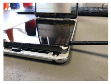
Once those screws have been taken care of you can then take the LCD out. Usually unless the device has been repaired before, the LCD will have some slight adhesiveness on the sides.
